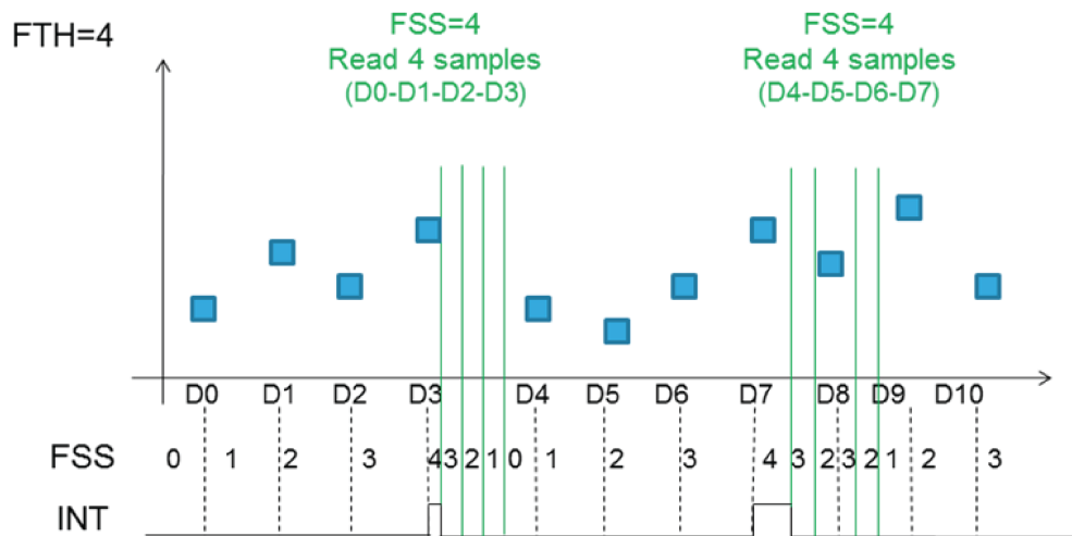
Figure 10. Continuous (dynamic-stream) mode
